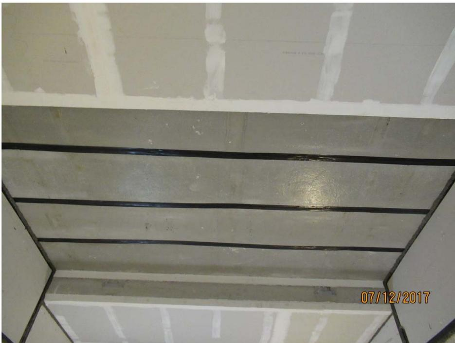
Figure 2 – Concrete slabs mounted in the test opening.
