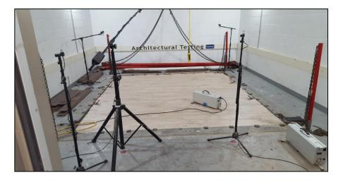
Source Room View of Test Specimen Installation
