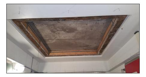
**Receive Room View of Test Specimen Installation**
