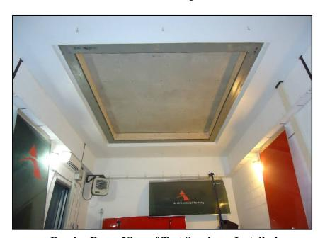
**Receive Room View of Test Specimen Installation**
