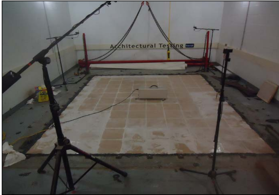
Source Room View of Test Specimen Installation
